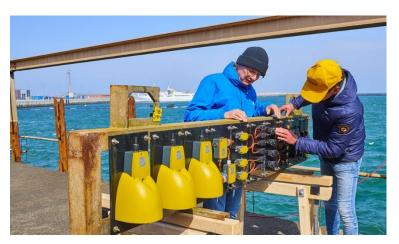
More realistic than laboratory tests: in a one-year outdoor exposure test, "oil & gas" switches were tested on the North Sea island of Helgoland, some of them in tidal water. The photo shows the condition of selected switches at "half time".
