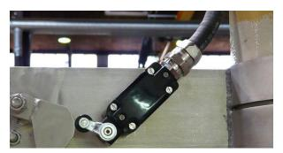
The position of the loading arm is monitored using a position switch which must be suitable for extreme environments.
