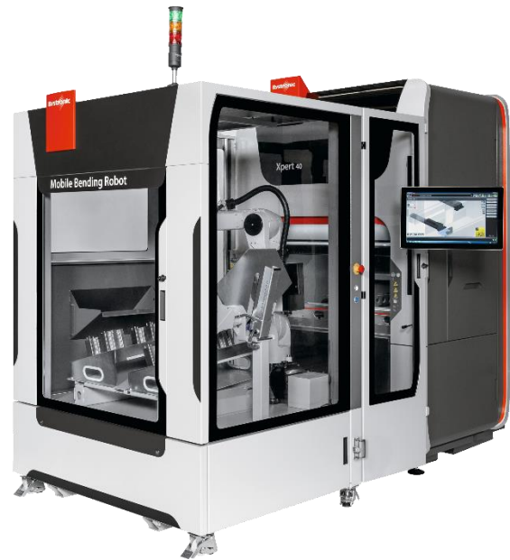
A mobile bending cell facilitates automation of a conventional press brake.
