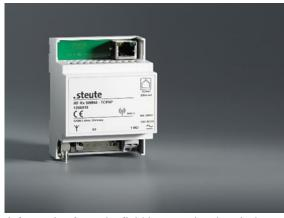
Information from the field is passed on by wireless receiver via a TCP/IP connection.
