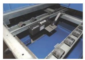
Wireless position switches from steute send a signal when a container is removed from a shelf.
