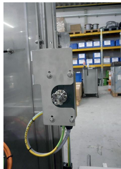
Fig. 4 The escape release is an option for the unlikely event that personnel become trapped inside the hazardous area.
